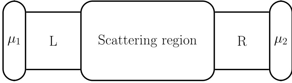
Figure 3.1: Schematic figure of a two terminal setup. \mu_1 and \mu_2 are the chemical potentials in the contacts. L and R are the left and right leads.
